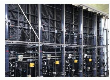
Pilot testing with filter columns to assess PFAS removal
